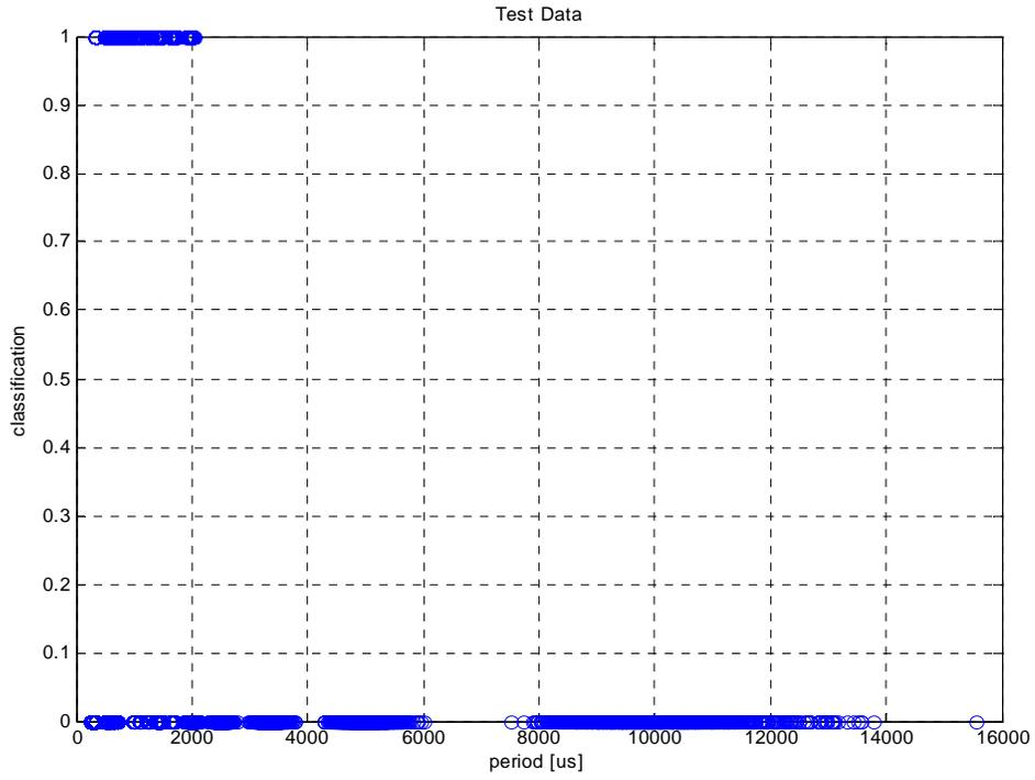
Figure 17. Test results for the DIG classifier vs. pulse period
