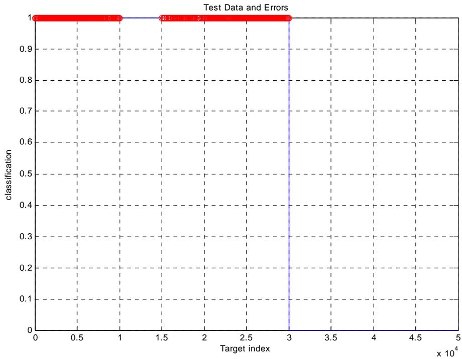
Figure 18. Error results for the DIG classifier. Red indicates an error.
