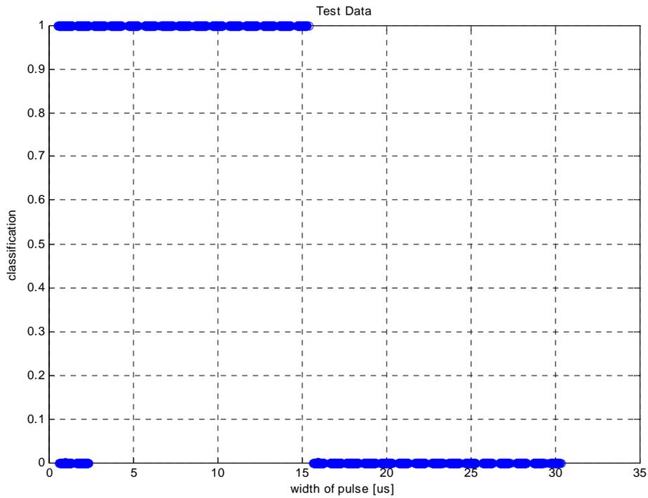
Figure 12 Test results for the NN classifier vs. pulse width.
