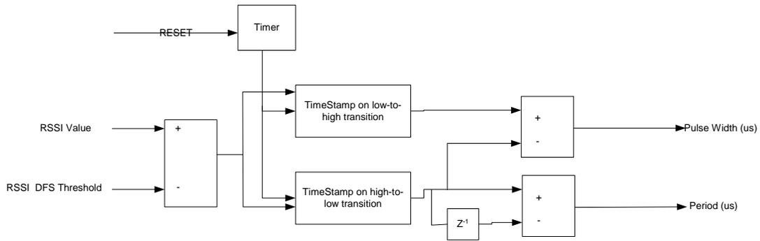
**Figure 2. Radar pulse characterization function.**
