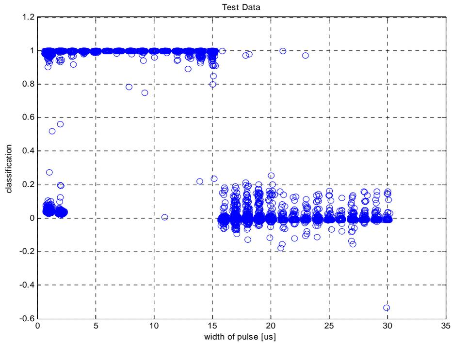
**Figure 9. Test results for the TDL-NN classifier vs. pulse width.**
