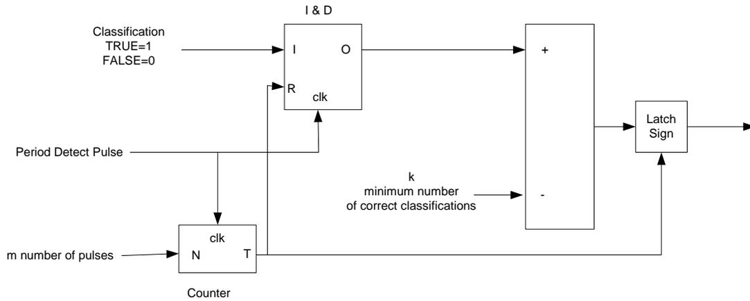
**Figure 5.** Summation block generates a TRUE output if more than “*k*” correct classifications are obtained out of “*m*” period detects.
