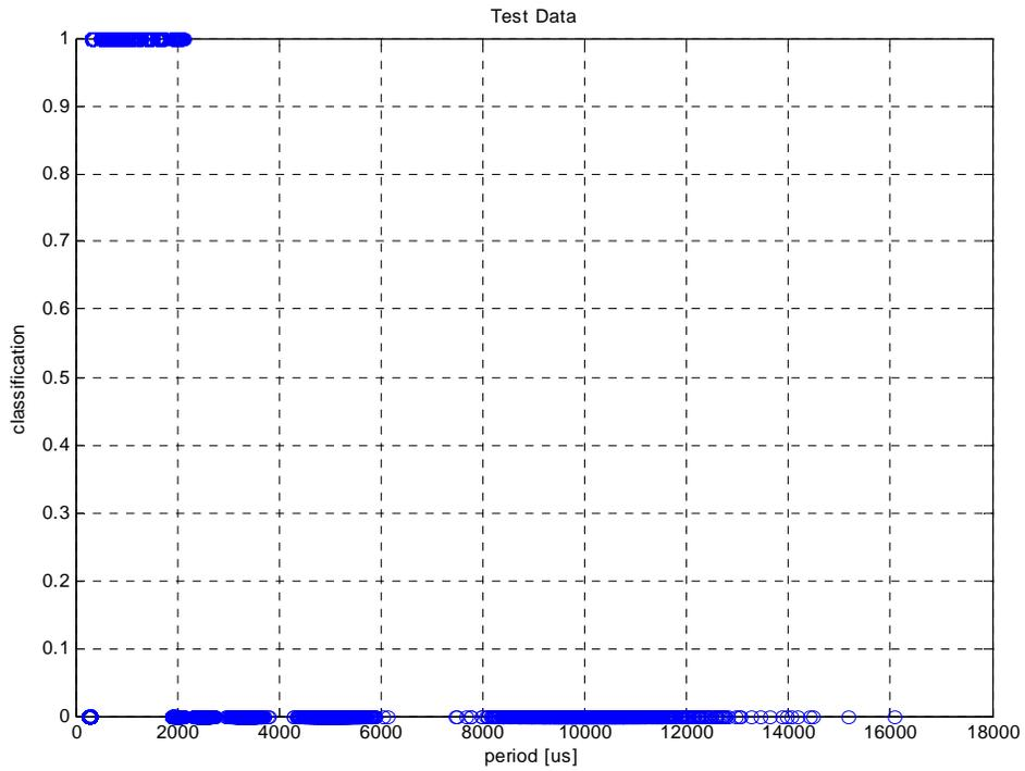
**Figure 13. Test results for the NN classifier vs. pulse period.**
